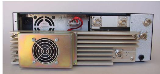
Figure 1. MX920 Rear Panel with Power Supply and Duplexer fitted. (RF Connecting cables not shown)
